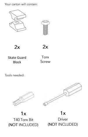
1. Position skate guard block in desired location & tighten to bench with the provided screw. Secured skate guard.
